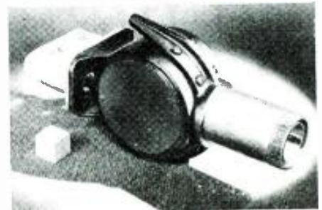
Fig. 8—A 20-kw magnetron, the W.E. 728-AJ, connected in parallel. These and other special types are either outmoded or have little general application and are interesting only from a purely academic viewpoint.
