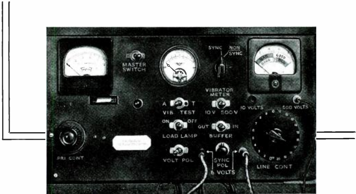
The front panel of the Carvalyzer. The A-eliminator inside the cabinet supplies the power.
