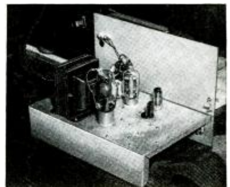
Rear view. Bias batteries are under chassis.
