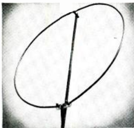
Mast supports the loop of exact center of top.
